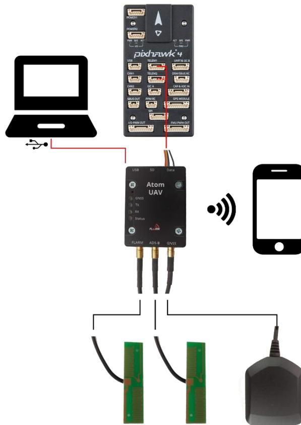
The diagram above shows a typical setup. Atom UAV is connected to a Pixhawk / PX4 flight controller, with a data interface and power supply. Optionally, power can be supplied through USB. Two FLARM/ADS-B antennas are connected to the FLARM and ADS-B RF connectors. A GNSS antenna is connected to the GNSS RF connector.
