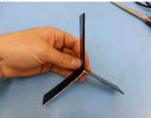
4. Apply double sided tape to the folded-out bottoms for subsequent installation in the airplane.
