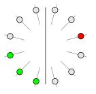
**Note:** Head-on ( $\pm 15^{\circ}$ ) traffic and collision warnings on Classic FLARM F6–F9 are indicated as shown in the graphic below (the traffic in this example comes from  $+5^{\circ}$  relative bearing).
