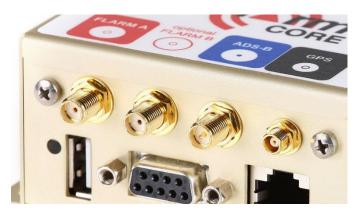
E-version devices (part No. FLAPFCnnE and FLAPFDnnE): FLARM A and B ports are standard female SMA connectors with a female center sleeve. ADS-B is a reverse polarity female SMA connector with a pin as a center conductor.
