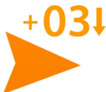
Large orange coloured aircraft symbol: this aircraft poses a threat of collision. The flight direction and height difference of the other aircraft are given to the nearest 100 ft, together with an indication of climb/descent. In this example: 300 ft higher, descending, flying from left to right.
