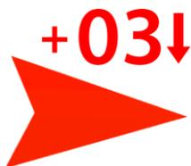
Very large red aircraft symbol: there is an immediate threat of collision. In addition, the display gives an indication of the vertical angle to the other aircraft. The flight direction and height difference of the other aircraft are given to the nearest 100 ft, together with an indication of climb/descent. In this example: 300 ft higher, descending, flying from left to right.
