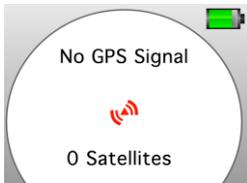
After acknowledging the disclaimer, the displays how many GPS satellites have been found. As soon as GPS reception is sufficient to give a worthwhile determination of position, the device then switches to normal operation.
