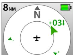
When on the ground, the 'radar' screen will operate provided there is adequate GPS reception. The screen image is then oriented to the North, symbolised in the screen by an 'N'.
