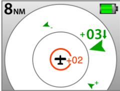
The circle turns orange, then red as the target closes in. In the example, the target is 200 ft above.
