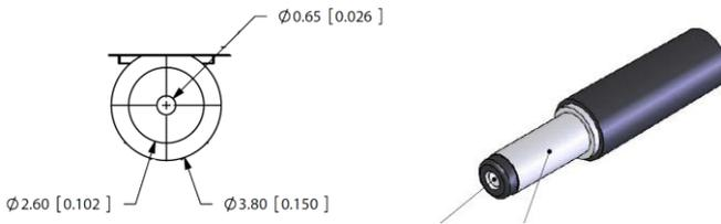
Supplied power must be 12 V DC nominal at 500mA (between 8V and 23V DC).
