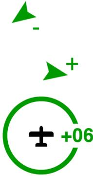
The small aircraft symbol gives the flight direction for distant aircraft. The sign indicates the relative position above or below you.
