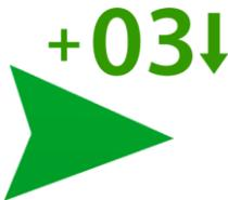
The large aircraft symbol always indicates the nearest aircraft and its relative track. Above the arrow (or below if the nearest aircraft is below), the relative height in steps of 100 ft and a small arrow showing climb/descent information is given. For example: 300ft higher, flying from left to right descending.
