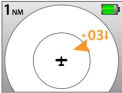
In dangerous situations, aircraft posing a threat are presented in orange or red, depending on the urgency of the threat. An acoustic warning is issued in addition to the optical warning.
